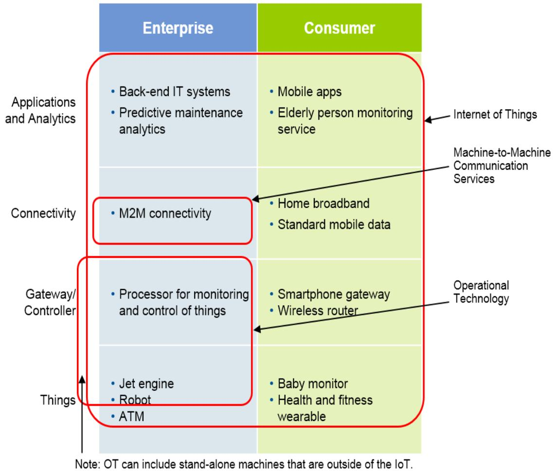
Figure 1. Relationship Between IoT, OT and M2M
